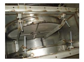
The catalyst's retention system is completely internal to the housing so there are no places for air to bleed into the housing to affect the performance of the catalyst. The system is designed to easily remove when it is time to replace the catalyst to get you back into operation quickly.
